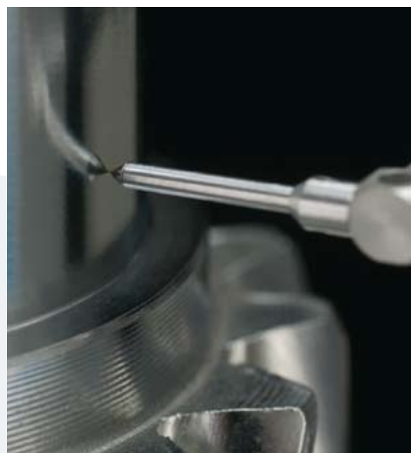
Twist measurement with a roughness stylus tip
