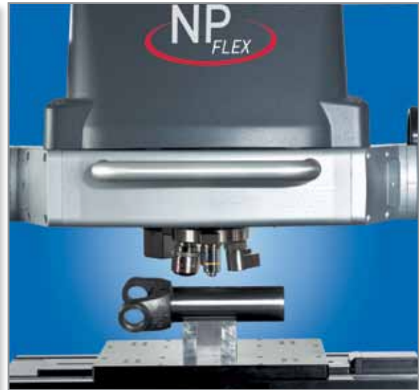
NPFLEX with objective turret measuring wear on yoke.
