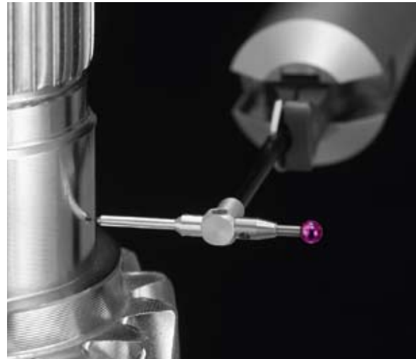
Twist measurement with a roughness stylus tip
