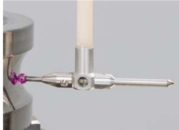
Form measurement with ruby ball
