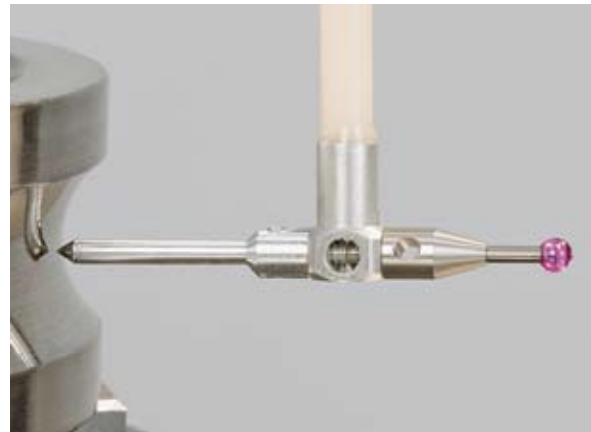
Roughness measurement with diamond tip
