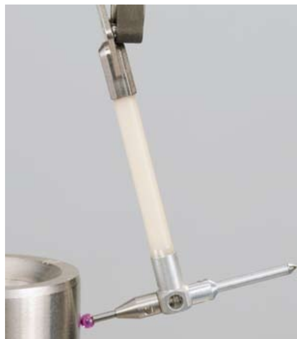
Collision protection by magnetic holder
